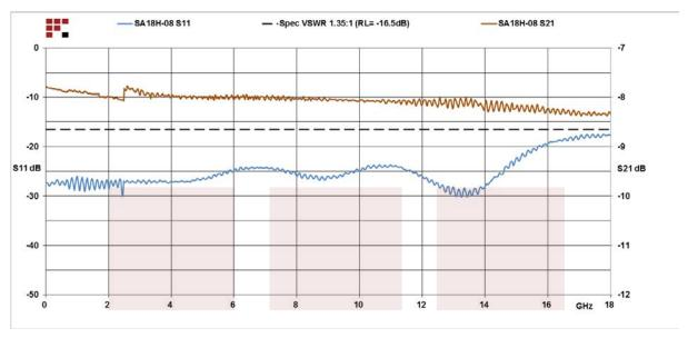
8 dB Fixed Attenuator SMA Male To SMA Female Up To 18 GHz Rated To 2 Watts With Stainless Steel Passivated Body from Fairview Microwave is in-stock and available to ship same-day. All of our RF/microwave products are available off-the-shelf from our ISO 9001:2008 certified facilities in Allen, Texas. Fairview Microwave is RF on-demand.
