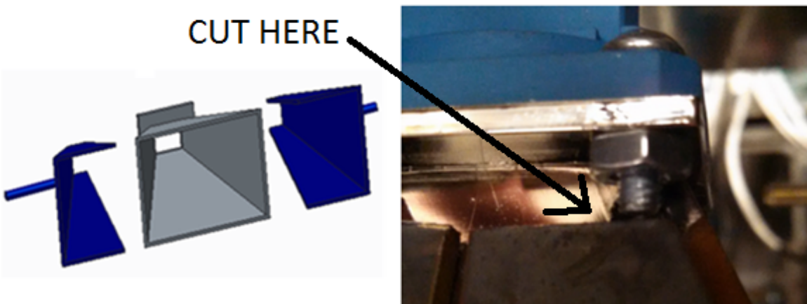
Figure 35: Horn Holder Adjustment
