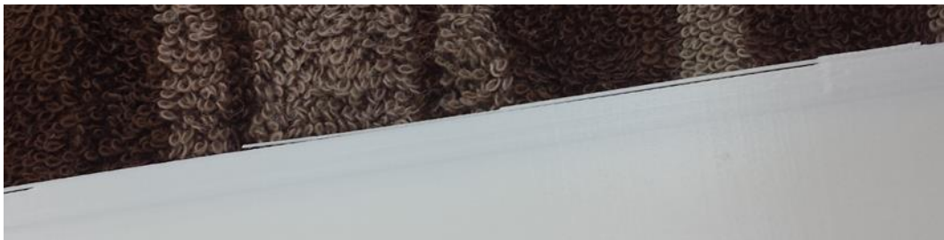
Figure 3. Chipping of 3D printed blades
