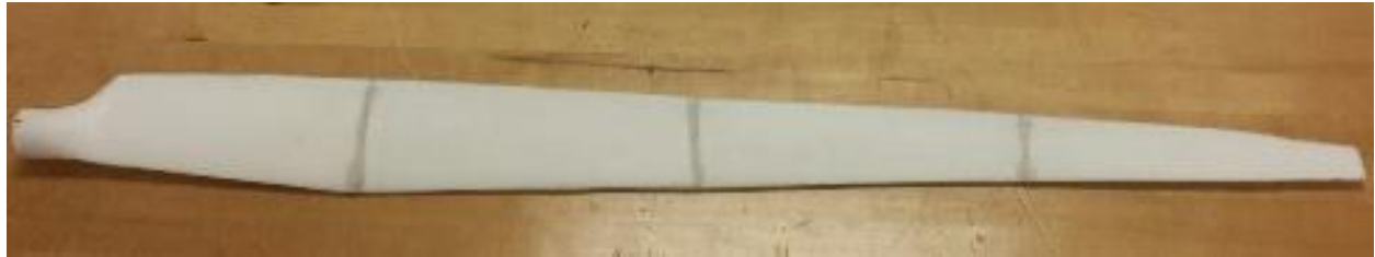
Figure 29. Fully fiber-glassed blades before paint
