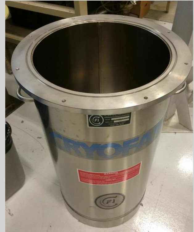
Cryofab CF 1424-F model cryostat that will be used in the project
