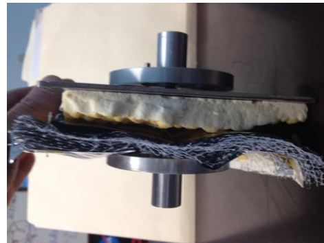
Figure 3: Layers of insulation currently in place on cryogenic tank
