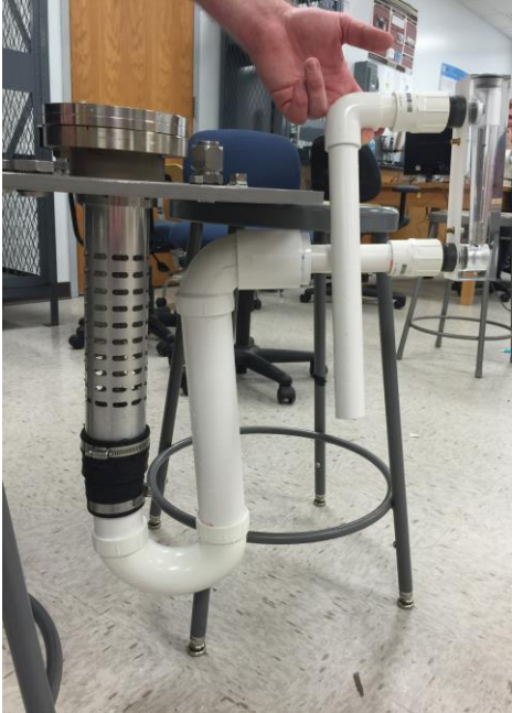
Figure 35: Setup for volumetric flow rate test
