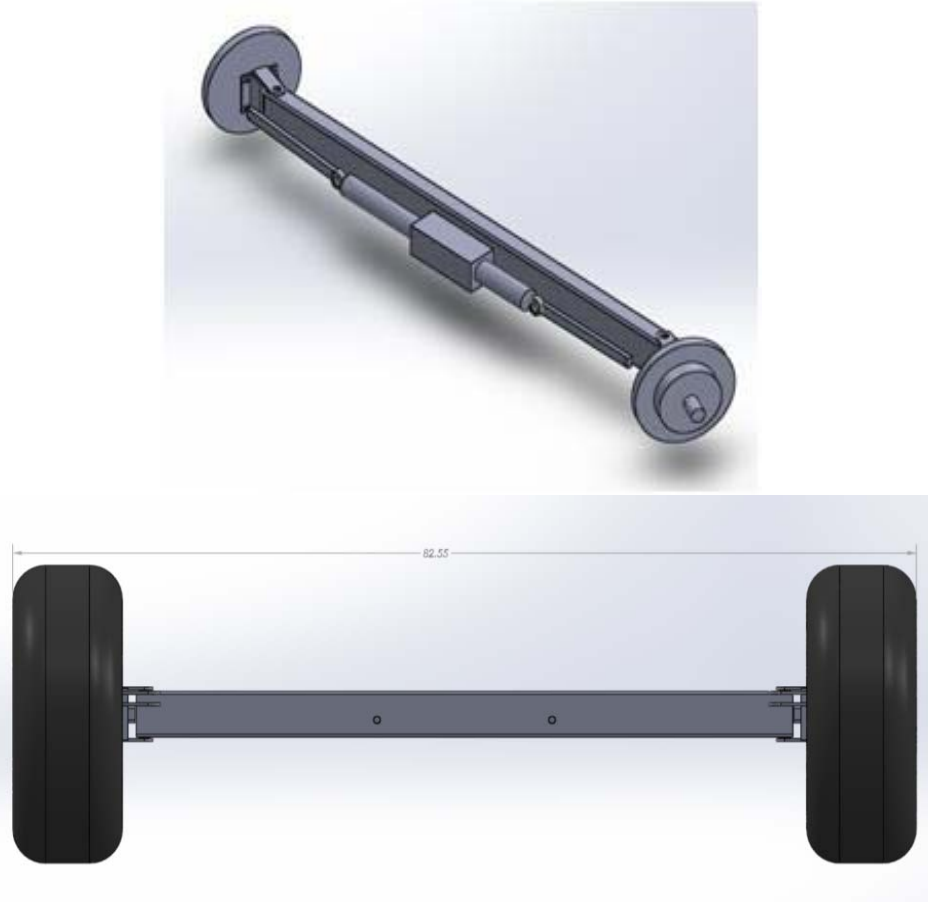
Figure 23. CAD renders of the finalized steering subassembly for the Pedibus including the appropriate dimensions.
