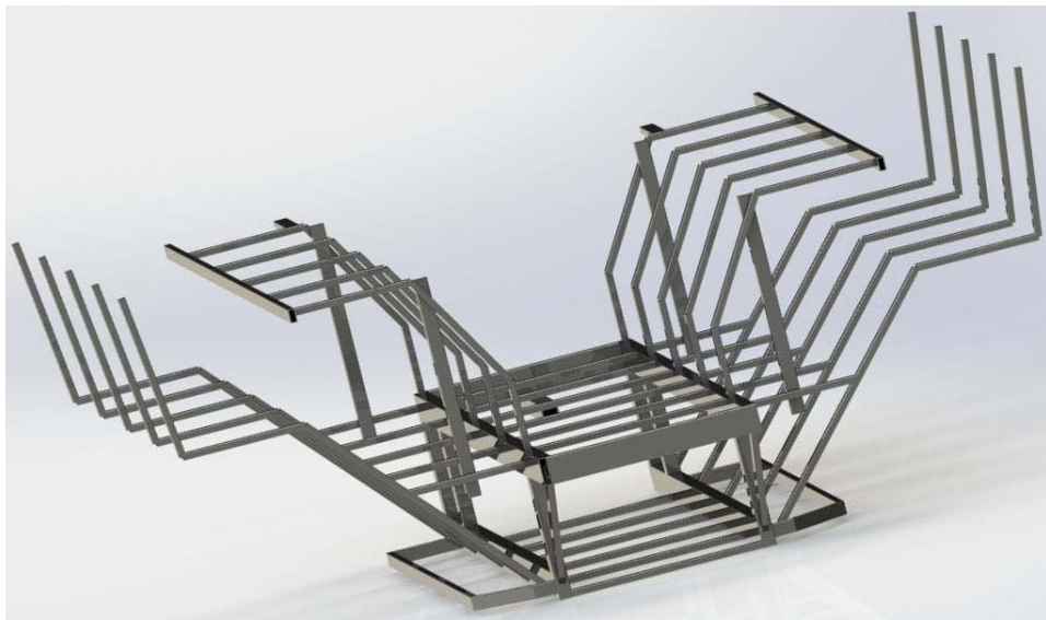
Figure 1. Box style frame render for the Pedibus.
