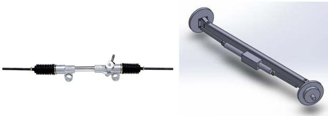
Figure 15. Rack and pinion steering CAD rendering and the actual rack and pinion mechanism purchased for the subassembly.
