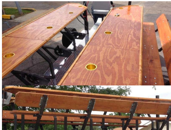
Figure 26. Finished wood components of the vehicle including the benched and the bar top.
