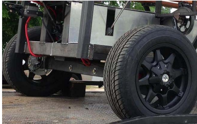
Figure 14. 16" trailer wheels utilized on the completion of the Pedibus.
