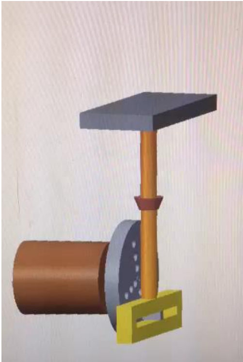
Figure 4. Scotch Yoke Design
