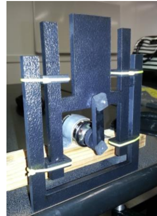
Figure. 9. Assembled prototype of crank slider design
