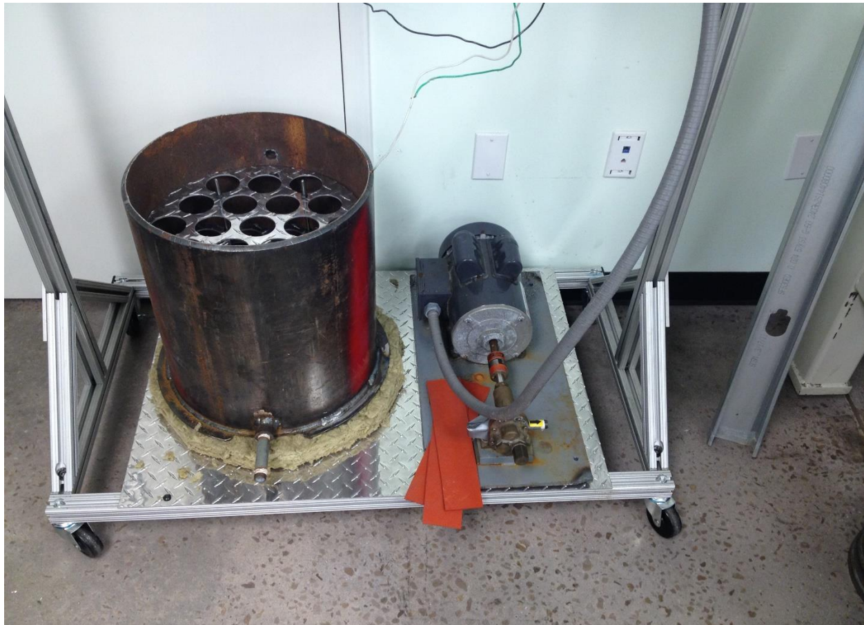
Figure 21 Tank with baffles frame installed
