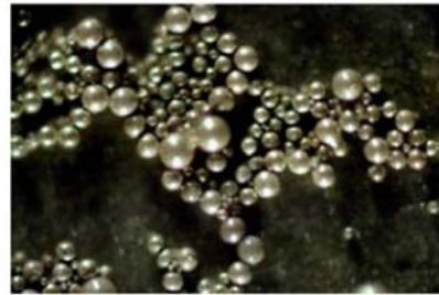
Figure 1. Optical microscope image of Stabilized Lithium metal powder.
