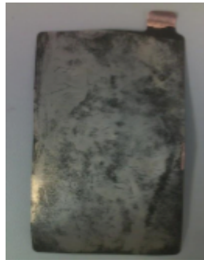
Image 3: Hard carbon electrode coated with SLMP.
