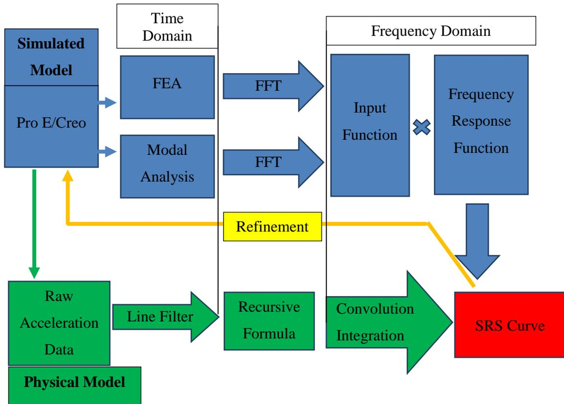
Figure 4- Flowchart depicting the methods of data processing
