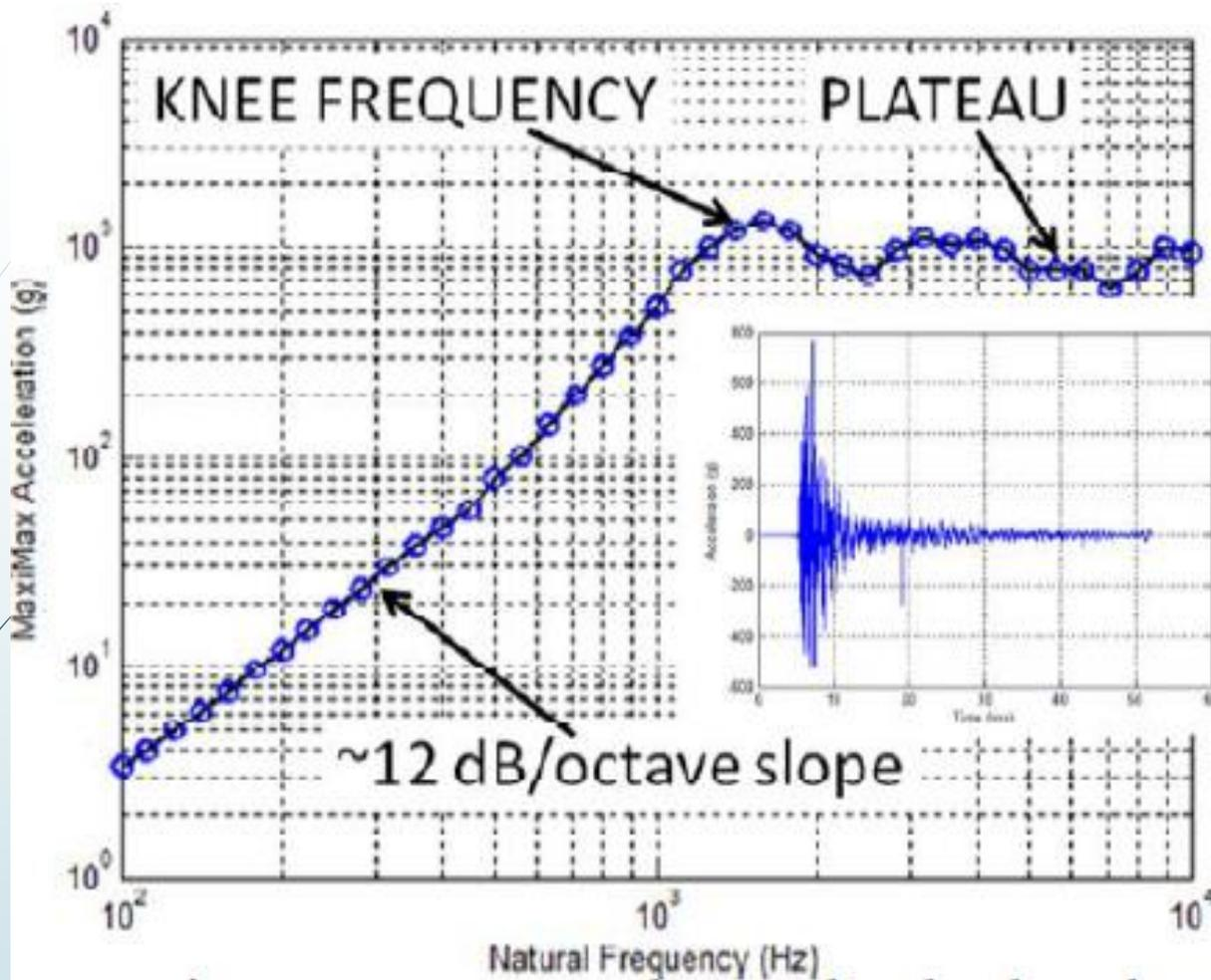
Figure 1 – Example of an SRS curve [1]
