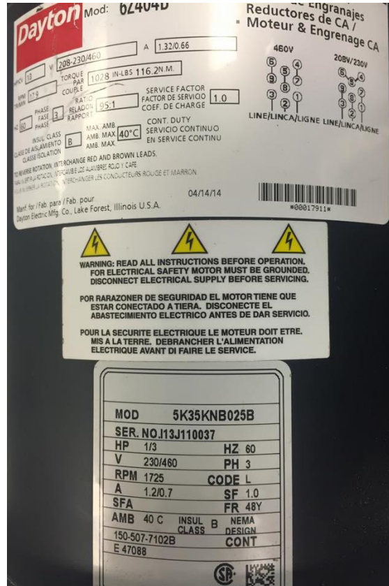
Figure 11: Motor baseplate information
