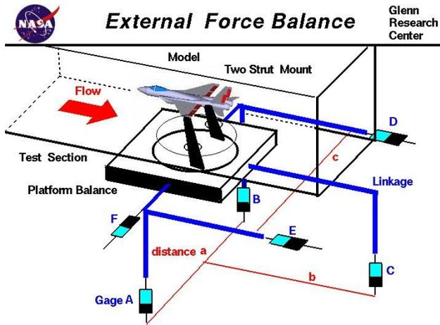
Figure 2: External Force Balance<sup>4</sup>
