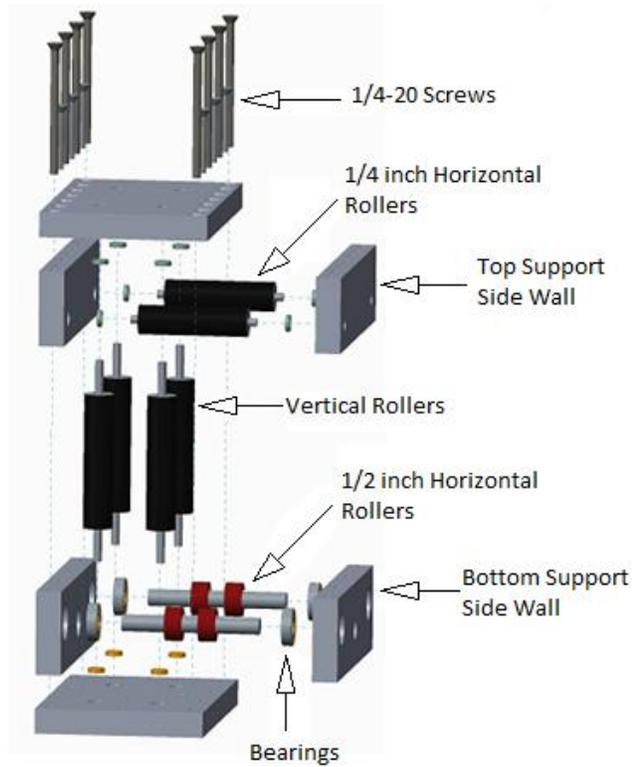
**Figure 3: Housing assembly**
