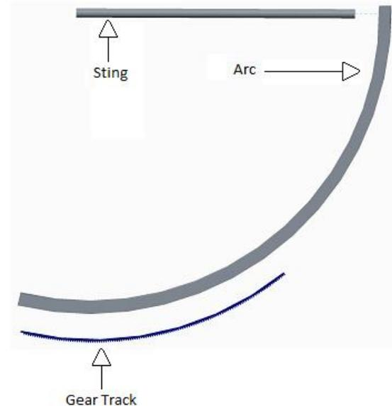
**Figure 2: Arc-sting assembly**
