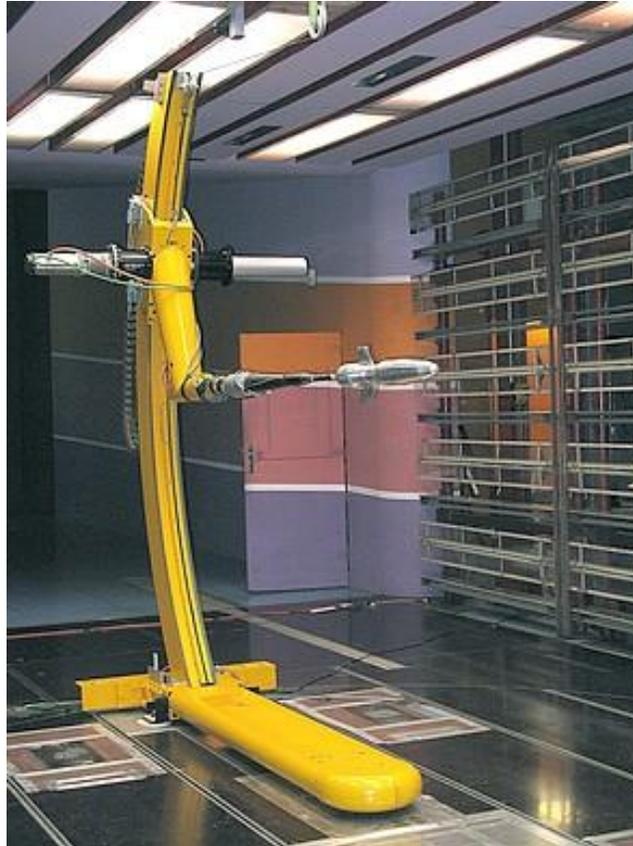
**Figure 5: Sting mount mechanism**
