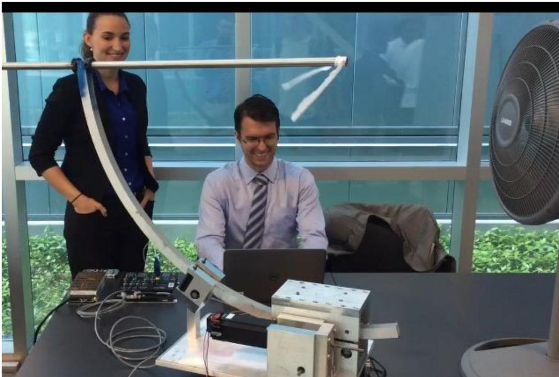
**Figure 33: Testing of pitch and yaw of mechanism unloaded**
