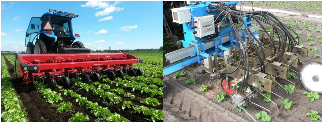
Figure 1. The Steketee IC Automatic Hoeing Machine 4
