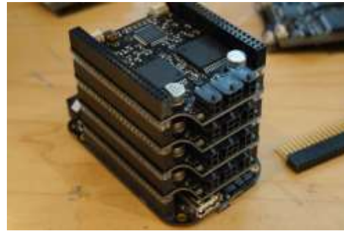
Figure 10. Dual Motor Controller Cape (DMCC) Mk.6 (Left), Device can stack to handle up to 8 motors (Right)
