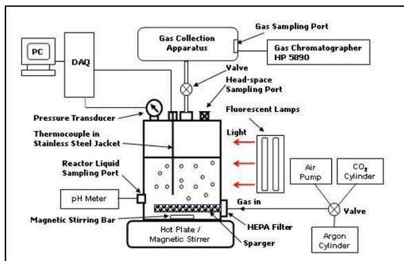
Figure 2: Schematic of a Photobioreactor.
