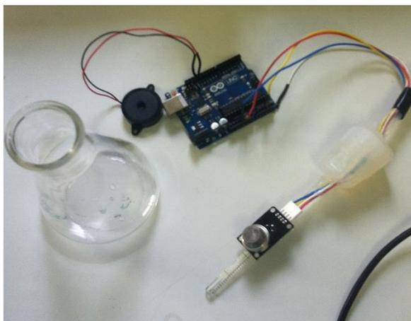
**Figure A:** Prototype of H<sub>2</sub> sensor system.
