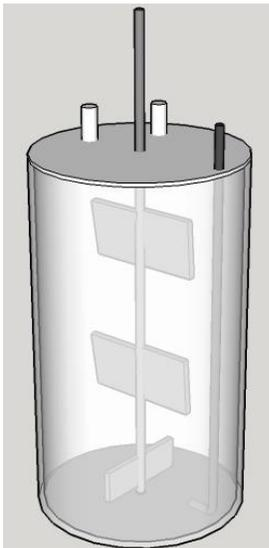
*Figure 6: Fermenter Bioreactor*
