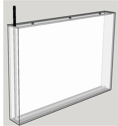
*Figure 5: Flat Plate Bioreactor*
