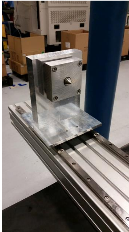
Figure 5: The live center assembly.
