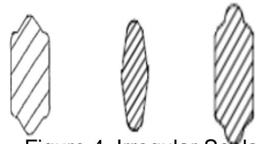
Figure 4: Irregular Seals - Diamond and Pseudo-Diamond Cross-sections
