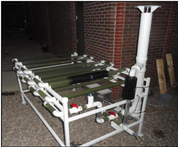
**Figure 2 shows the Photobioreactor created last year. It incorporated sensors to monitor the microalgae growth. (Senior Design Project)**
