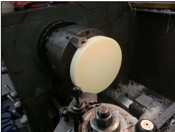
Figure 8 - Turning nest plate to size on lathe
