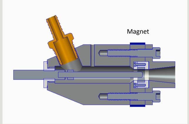
We will use an electromagnet to vary the magnetic field and optimize the thruster performance, then order permanent magnet based on the tested magnetic field strength. The generated magnetic field at the center is:
