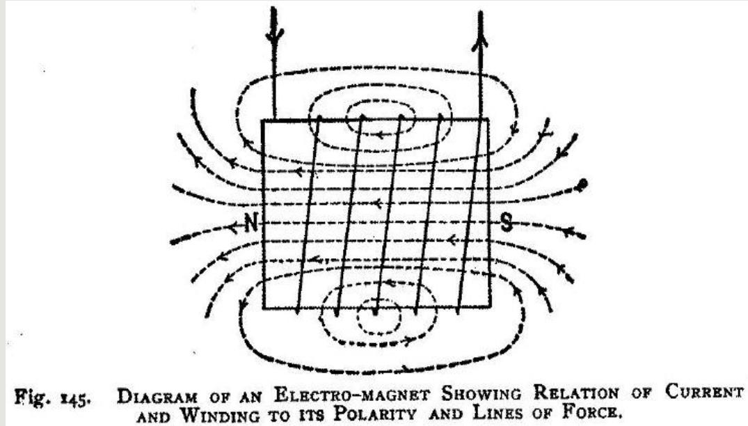
Fig. 145. DIAGRAM OF AN ELECTRO-MAGNET SHOWING RELATION OF CURRENT AND WINDING TO ITS POLARITY AND LINES OF FORCE.
