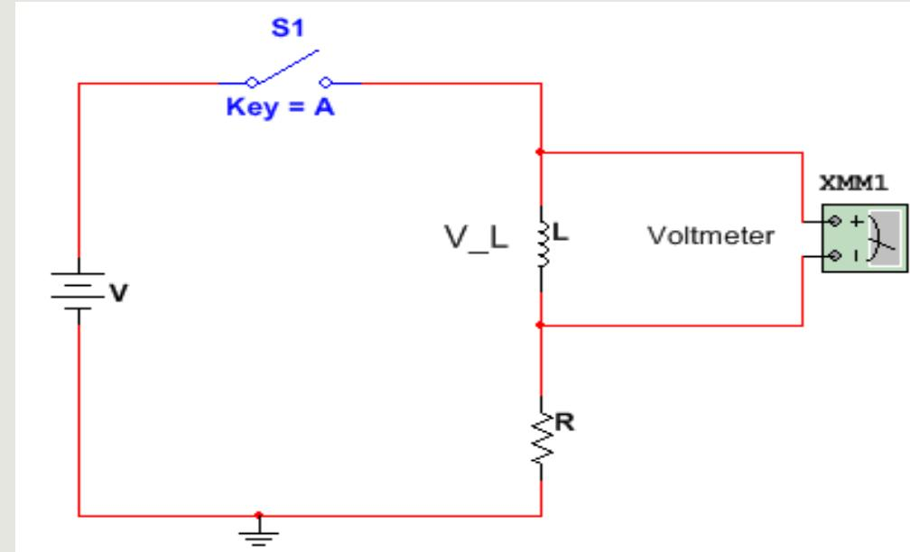
$$\text{When the switch opens: } V_L = L \frac{di}{dt} = L \frac{I - 0}{dt}$$
