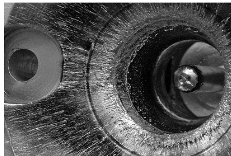
Figure 70: Anode Material Loss
