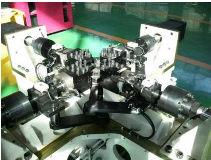
Figure 5: Tensile Machine Pulling Along Two Axes
