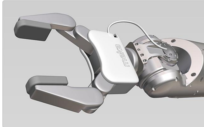
Figure 21 -- CAD Model of a Pincer Design
