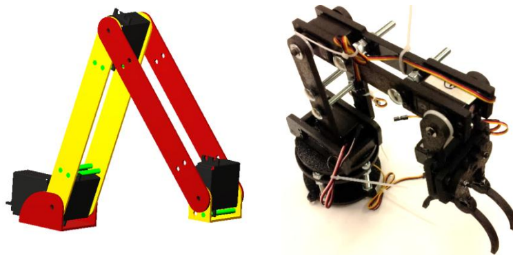
Figure 35 -- Initial Design CAD and Prototype
