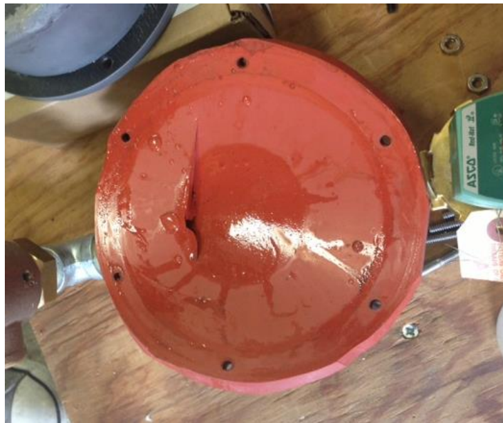
Figure 10: Ruptured Diaphragm after Steam Test
