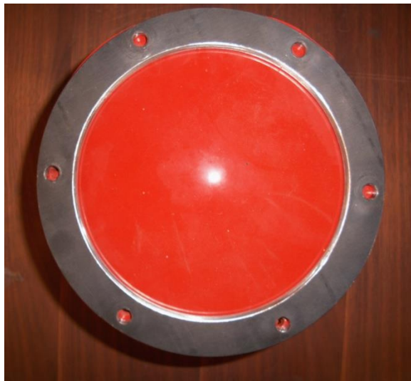
Figure 8: Initial Pressure Test of Membrane
