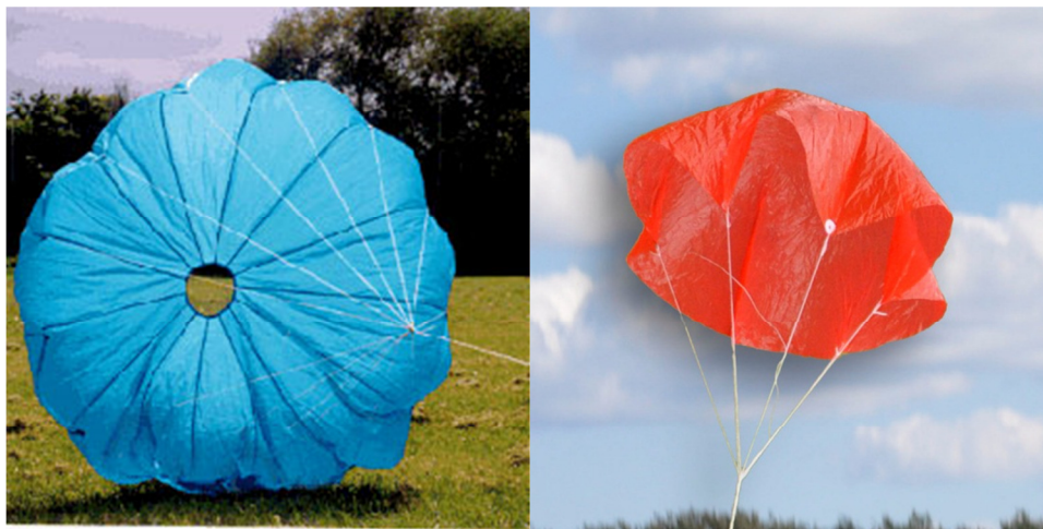
Figure 4 shows a true dome shape round parachute on the left and a flat round parasheet on the right.
