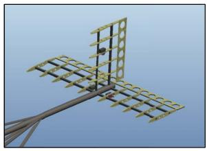
The tail section was made up of three components. The tail connector was made up of a very rigid carbon composite tube, which would transfer the moment induced by the control surfaces on the tail. The elevator and rudder were both constructed in the same fashion as the wing, but used a different laser-cut airfoil anddremmel-cut spar size. The elevator was constructed by running two single carbon
