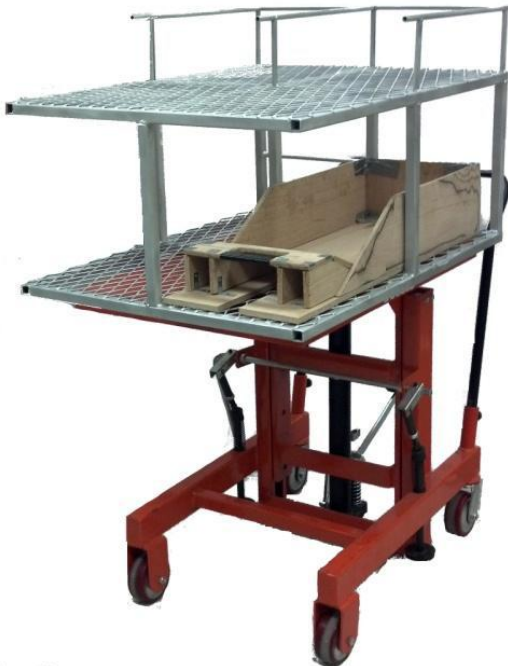
Figure 1 – The existing cart prototype designed by the 2012 Senior Design group.
