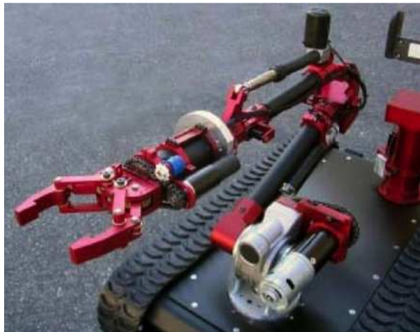
Figure 13: An example of a pincer-gripper. Image obtained from the Science in Seconds Blog.
