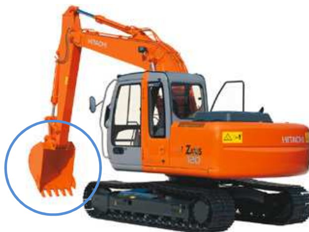
Figure 14: An excavator with the item of interest, its scoop, encircled.
