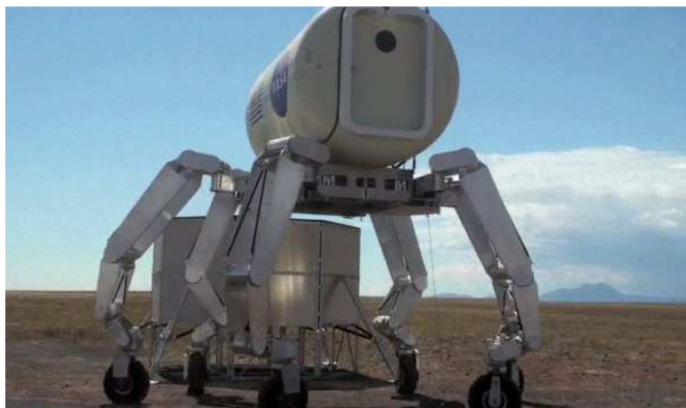
Figure 1: NASA's Athlete Rover carrying a prototype habitat module. Image from the NASA Jet Propulsion Laboratory website.
