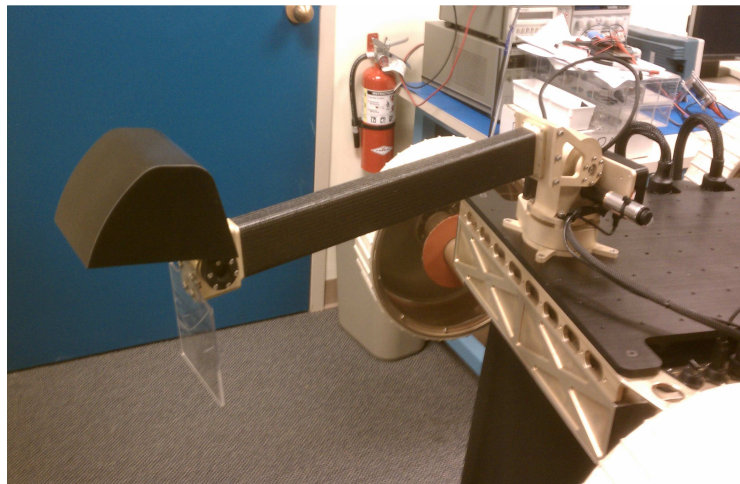
Figure 5; WPI's arm and claw design for the 2012 competition.
