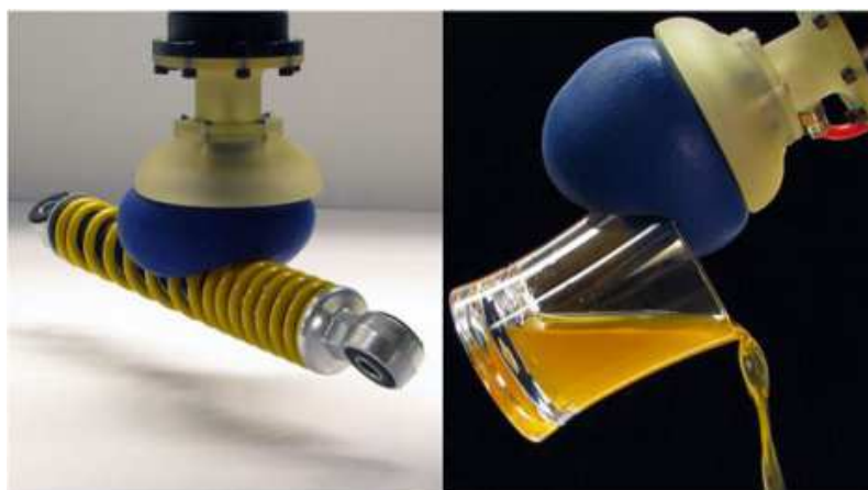
Figure 16: The universal gripper conforms to the shape of any object it is lifting to allow for a delicate yet firm grasp
