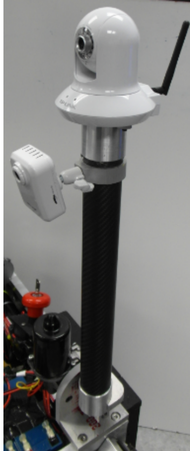
Figure 17 - Camera boom mounted on the rear left corner of the rover.
