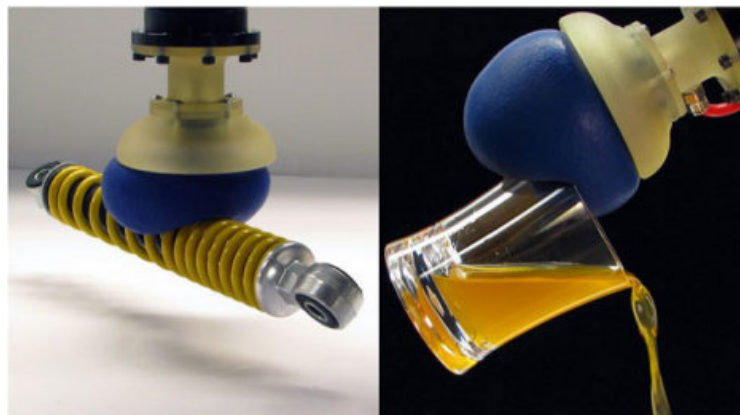
Figure 52: The universal gripper conforms to the shape of any object it is lifting to allow for a delicate yet firm grasp
