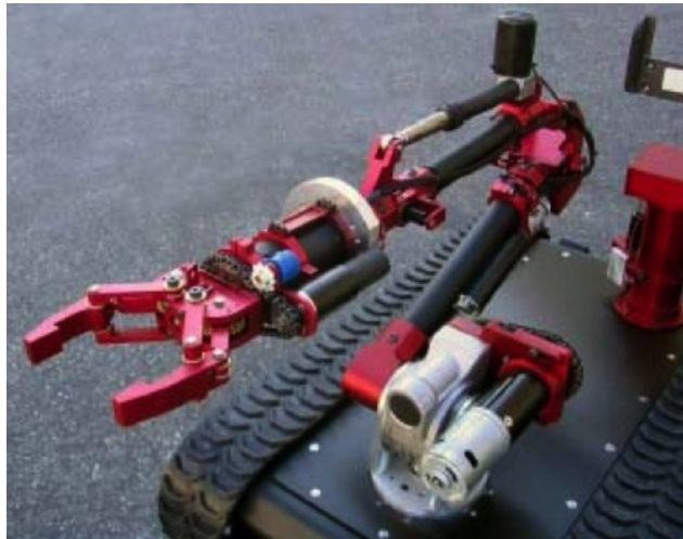
Figure 49: An example of a pincer-gripper. Image obtained from the Science in Seconds Blog.
