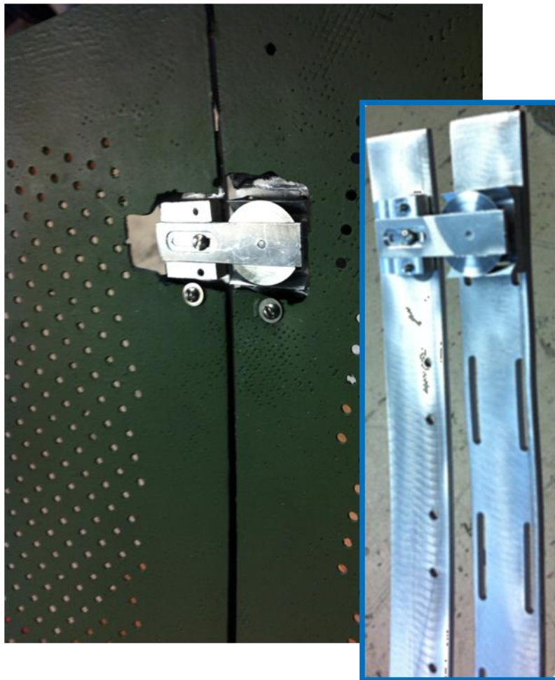
Figure 26. The support structure subsystem with detail of armature bracket (left) and v-block bracket (right).
