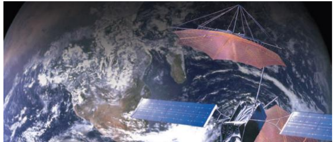
Existing Approach: Unfurlable Mesh-Rib Reflector
