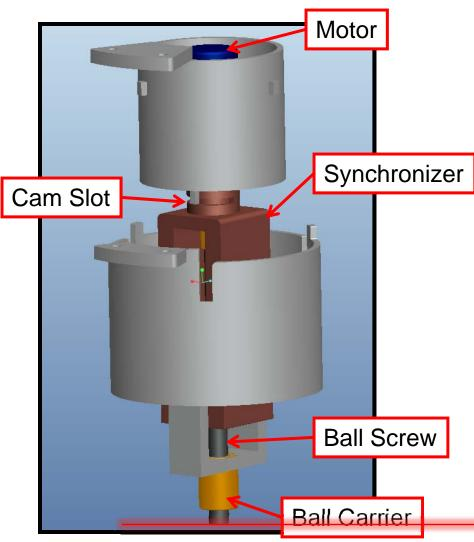
Motor shaft initially fixed to synchronizer
