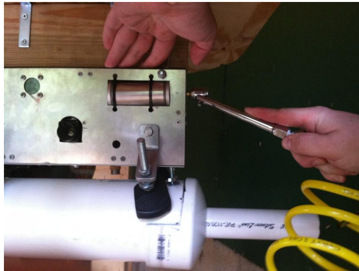
Figure 44- Filling the BRU using Schrader Valve
