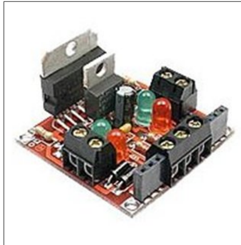
Figure 31: L298 Dual H-Bridge Motor Driver for the Thrusters
