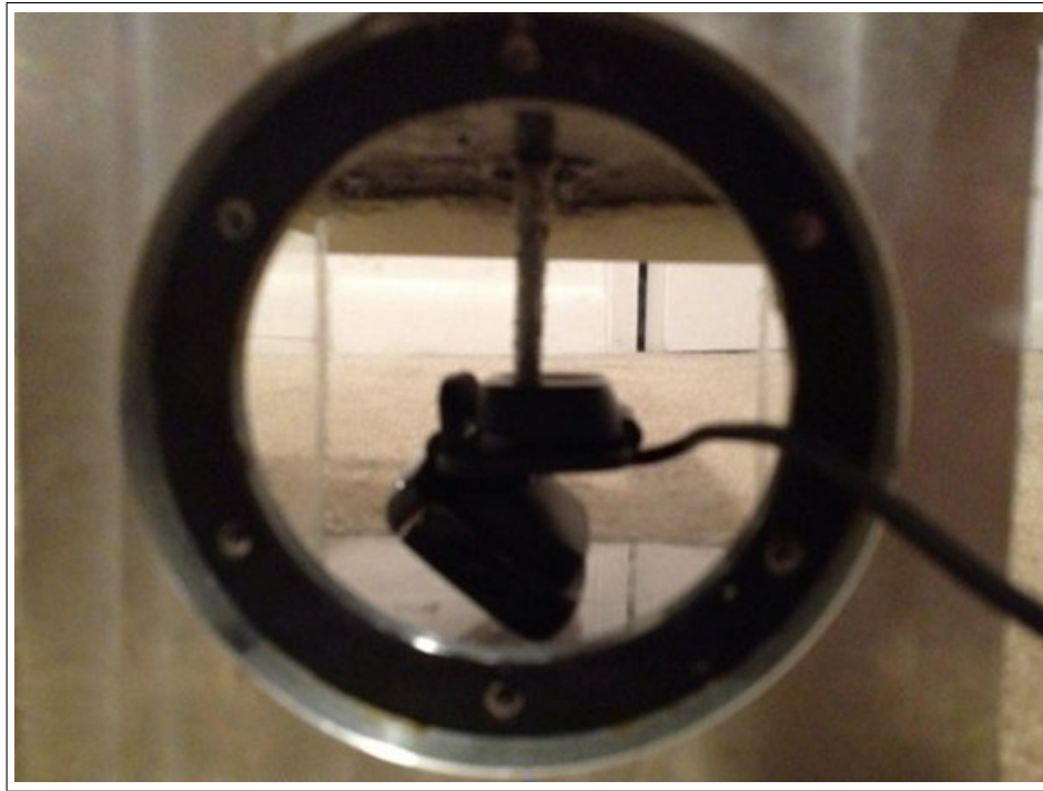
Figure 21: Endcap View of Logitech C615 inside Camera Enclosure
