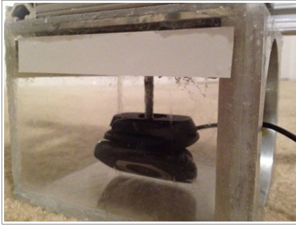
Figure 20: Front View of Logitech C615 inside Camera Enclosure
