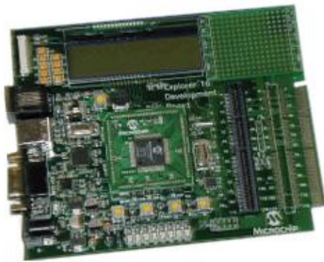
Pic Development Board W/ Programmer - Alpha-numeric 16x2 LCD Display
