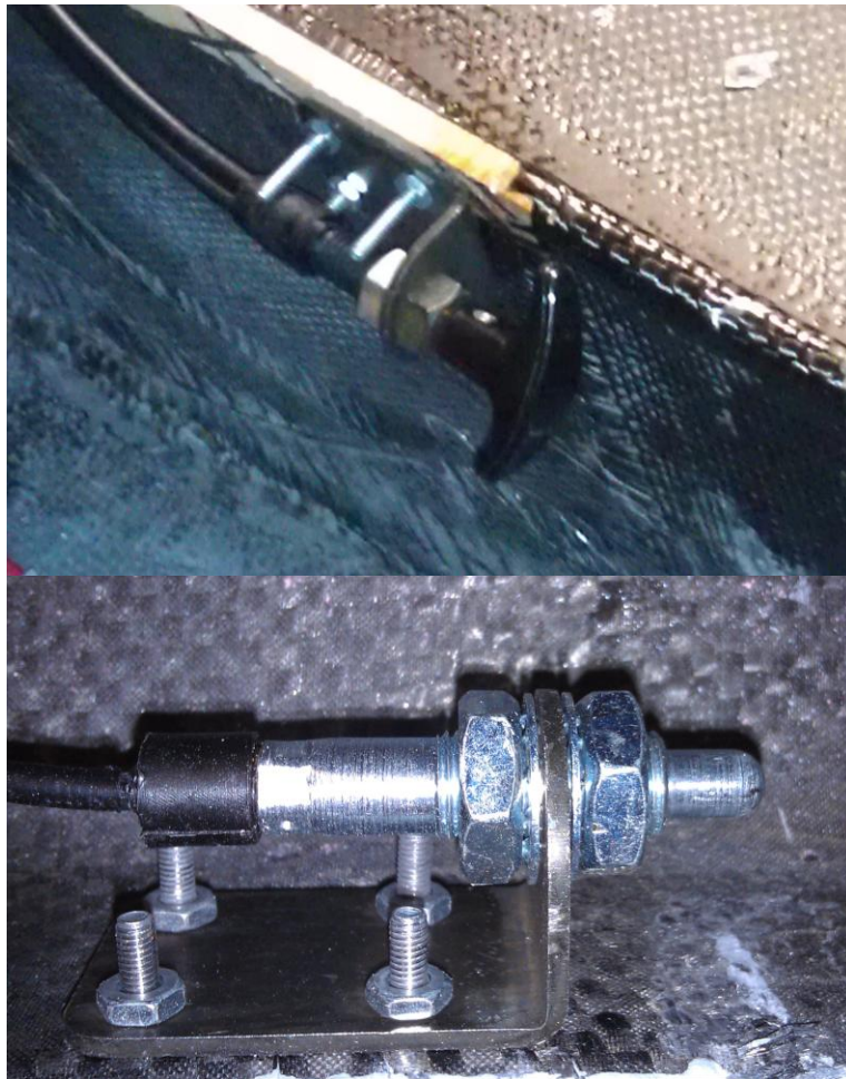
Figure 39 - Top: Latch actuation handle. Bottom: Latch point.
