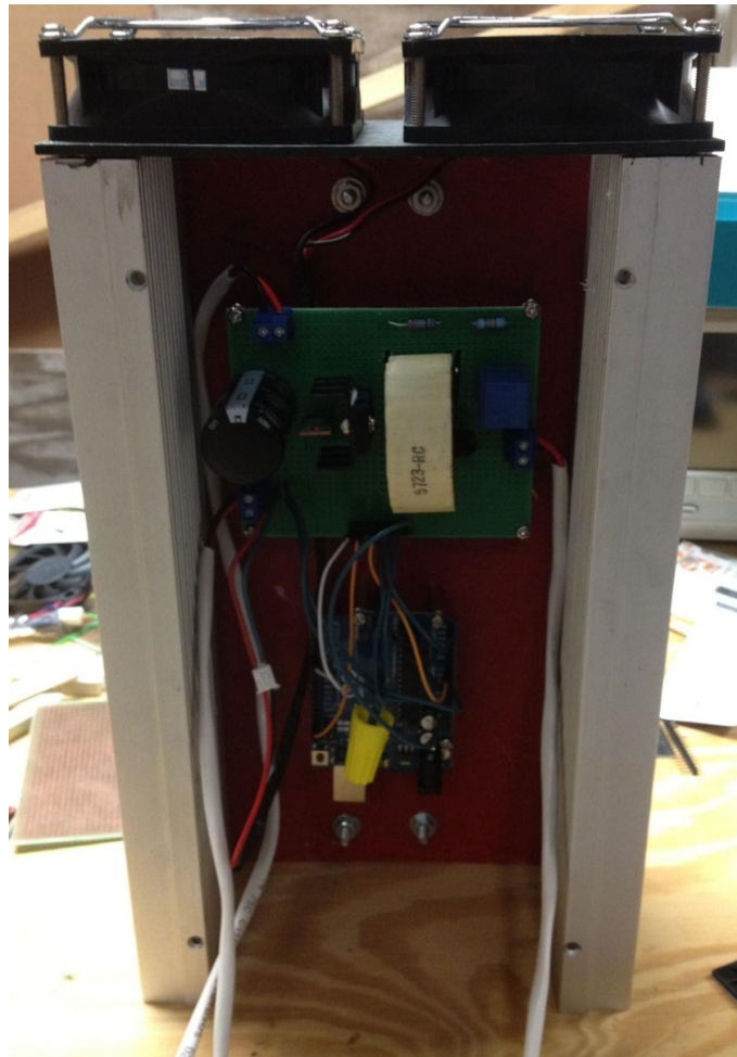
Figure 32 - Final construction of boost converter and controller
