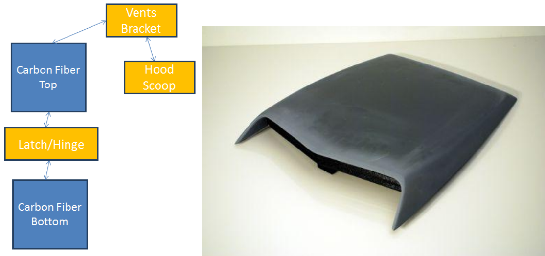
Figure 42 shows the top level diagram for the hood scoop. On the right is the first concept design shape.
