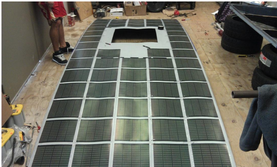
Figure 23 - Implementation of design placement.
