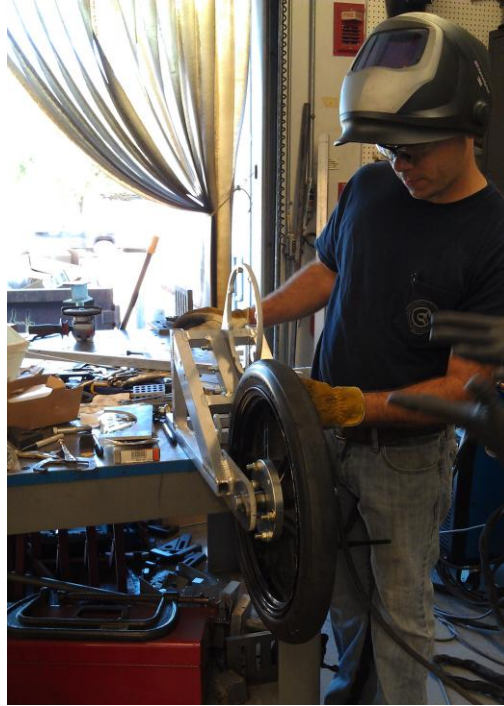
Figure 37 - Jeremy (machine shop manager) about to weld the motor bracket on the rear arm.
