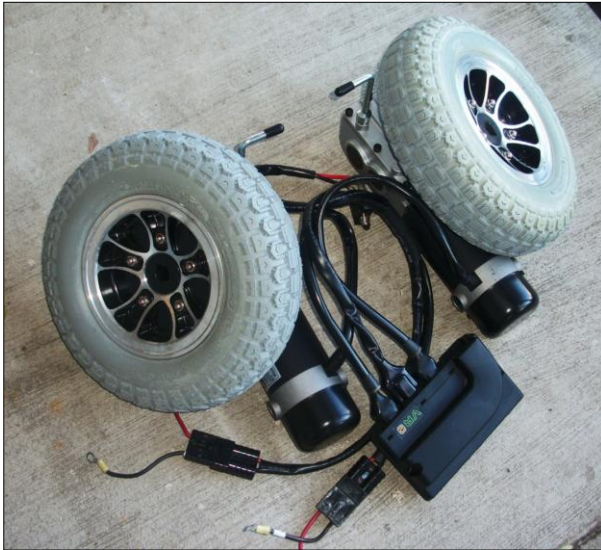
Figure 19: Motion Tech motors and tires
