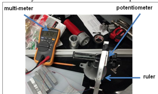
Figure 34: Setup for potentiometer Test
