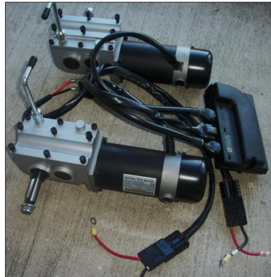
Figure 18: 4600 RPM Motion Tech Motors
