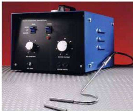
Figure 7 - Air flow tracer
