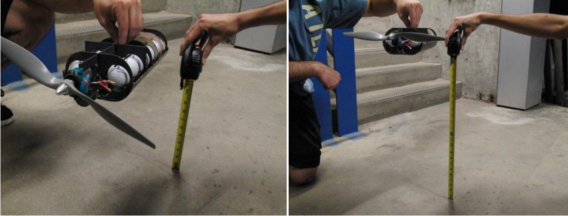
Figure 8.4: Landing Platform Drop Testing – 1 ft drop (left) and 2 ft drop (right)
