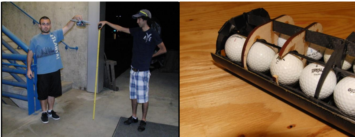
Figure 8.5: Landing Platform Drop Testing – 5 ft drop (left) and wooden bulkhead fracture (right)
