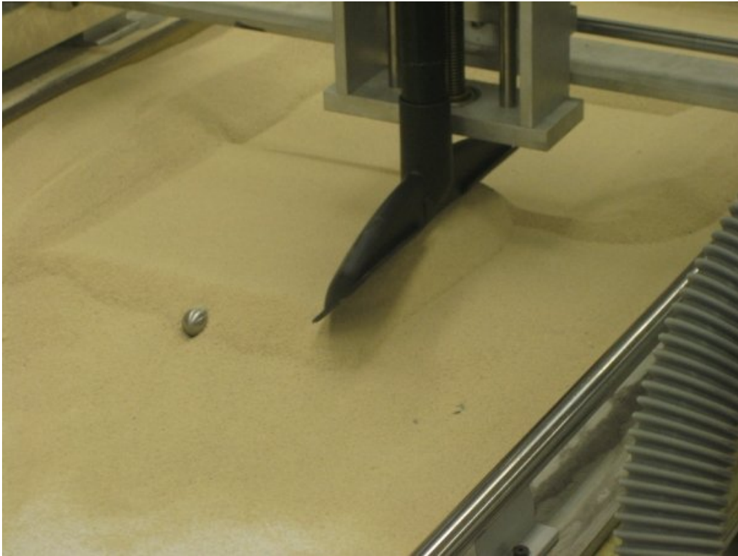
Figure 46: Standard Shop Vac Tip Design
