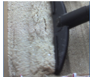
Figure 28b: Sand accumulation on front tip with an expansion
