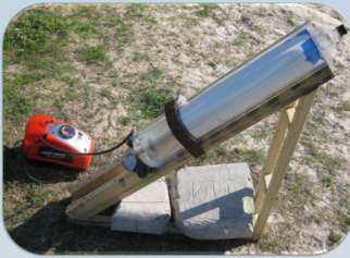
Stage 1 – Pressure Reservoir Loaded
