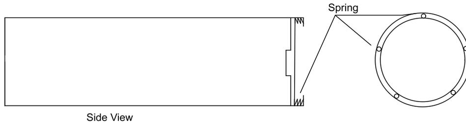
Figure 30 – Dampening System Concept
