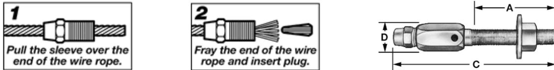
Figure 32 – Wire Anchor for Stopping Mechanism
