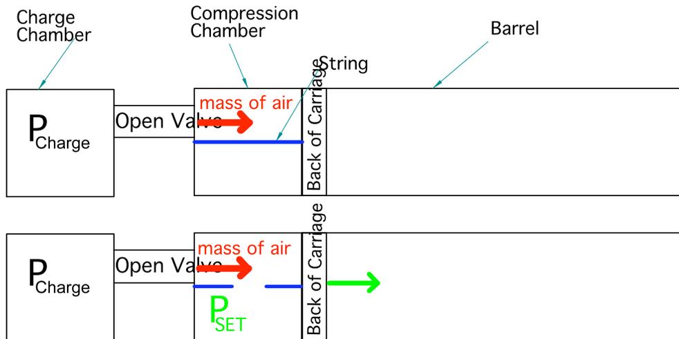
Figure 21 – Breaking String Method
