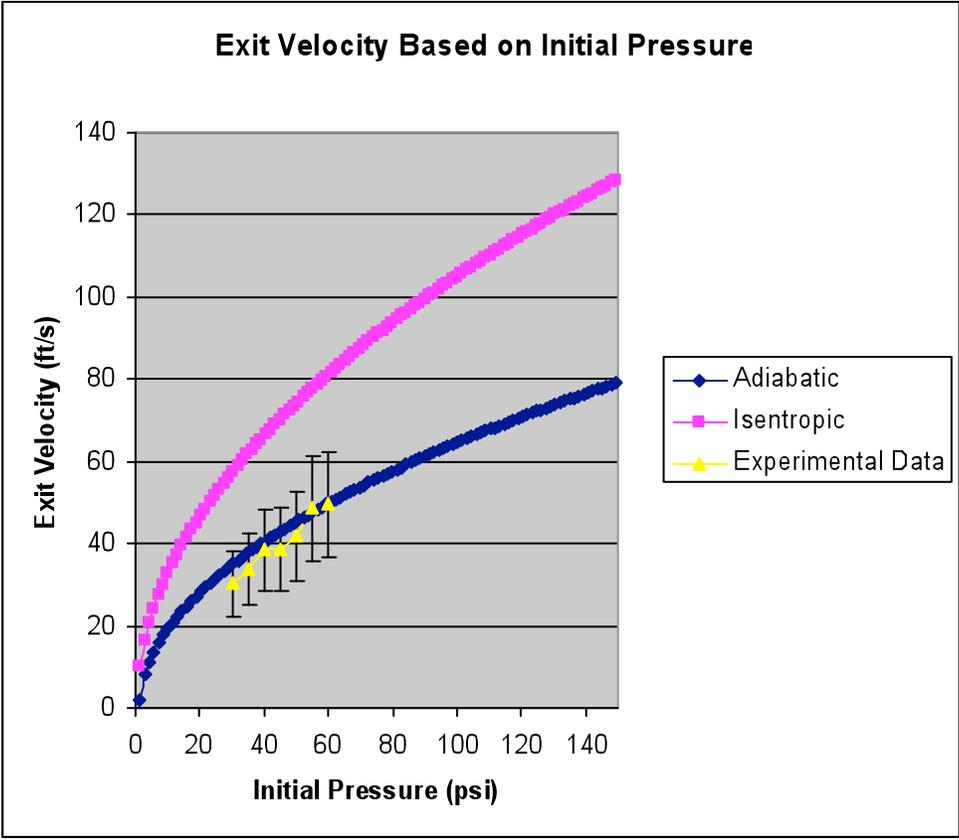
Exit Velocity Based on Initial Pressure
