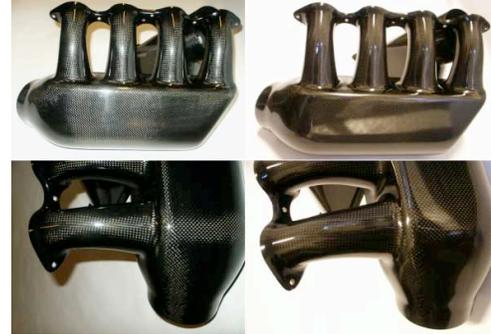
Figure 14– BMW's new Carbon Fiber air box
