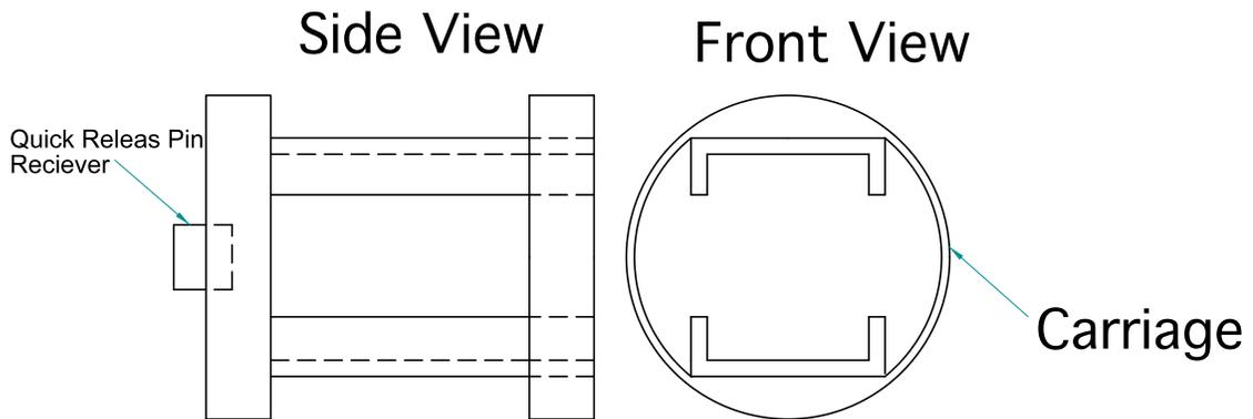
Figure 20 – Carriage without Insert
