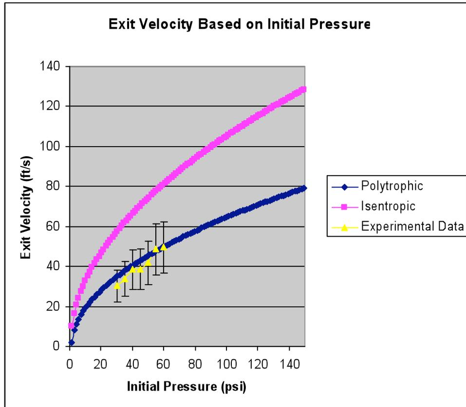
Figure 49– Exit Velocity Based on Initial Pressure
