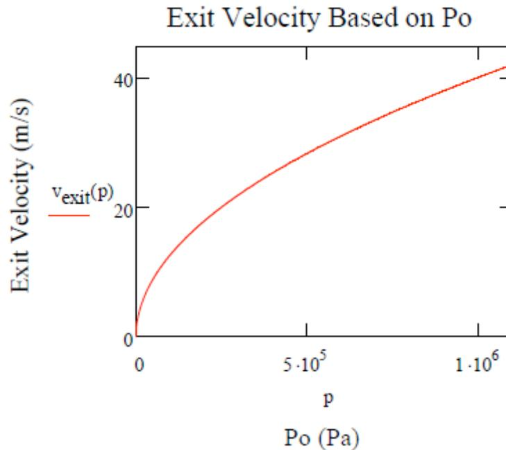
Figure 34 – Exit Velocity Based on  $P_0$
