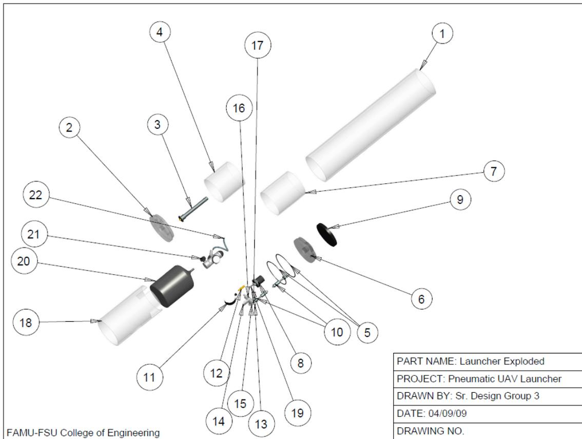
Figure 44 – Exploded View of Prototype
