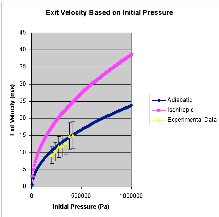
Exit Velocity Based on Initial Pressure
