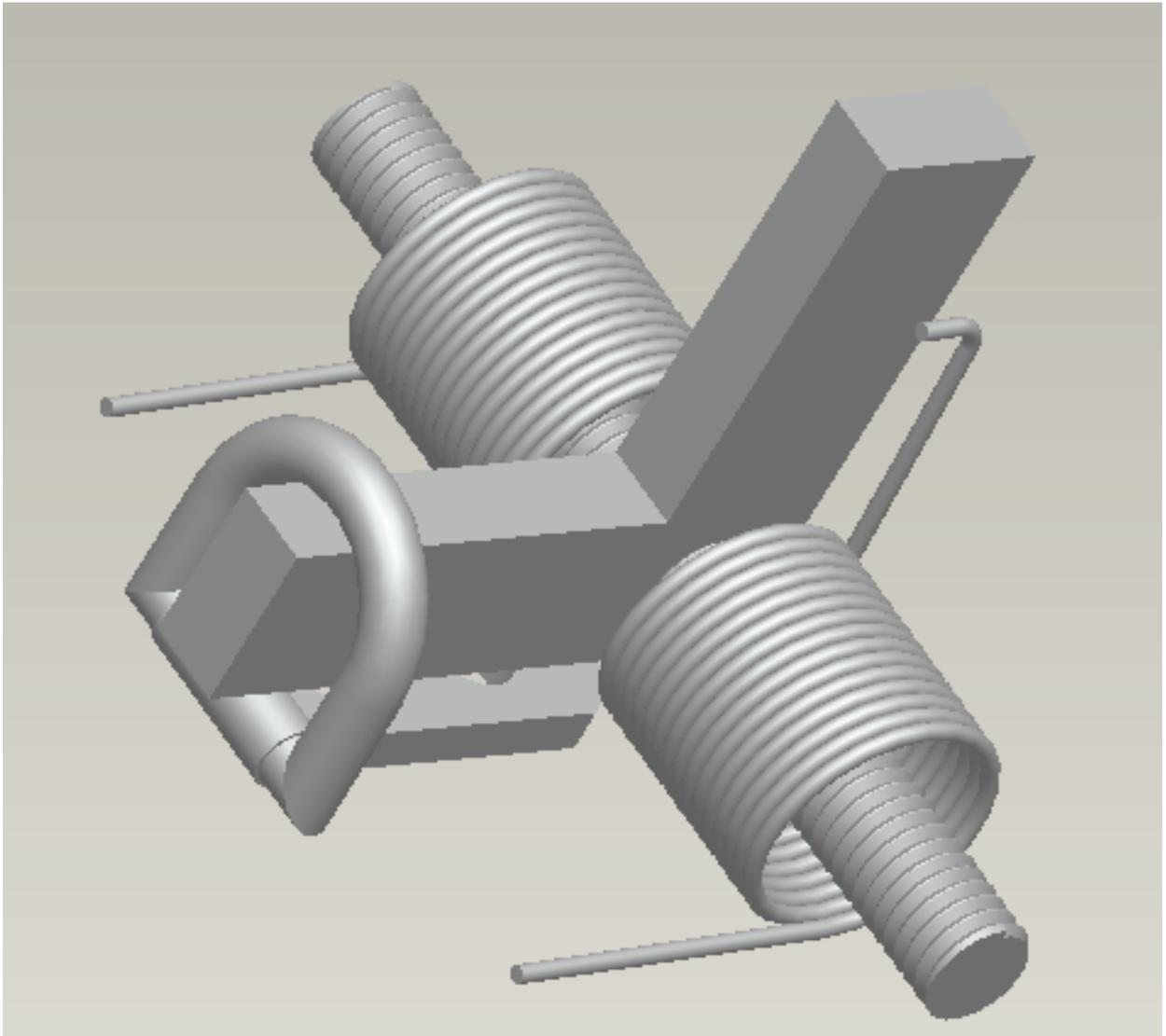
Trigger Mechanism Assembly
