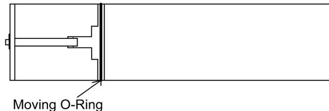
Figure 25 – Moving O-Ring Concept
