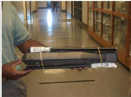
Figure 4– side view of the UAV (wings retracted)
