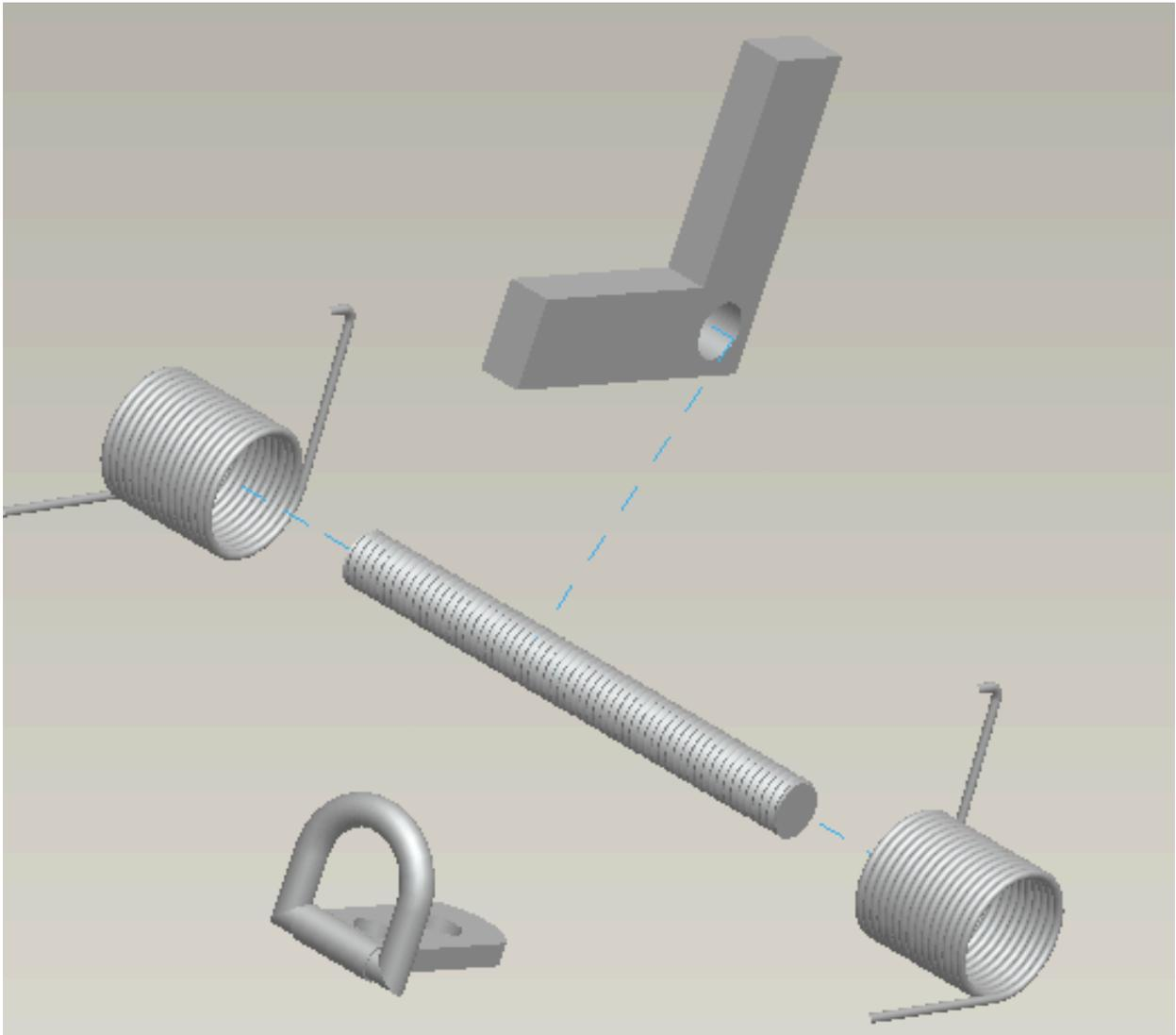
Trigger Mechanism Exploded View
