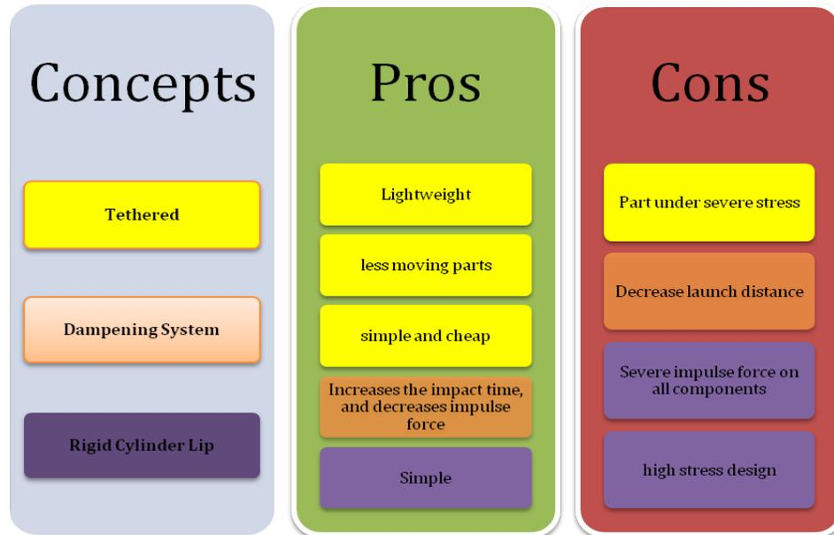
Due to weight restrictions, the dampening system and the rigid lip cylinder were ruled out (Table 6). The cable was also a more simple design and less costly than the other two designs. The rigid cylinder lip has the potential to inflict damage on both the carriage and itself. Once the team decided to use the cable, one needed to be found that would satisfy all of the requirements.
